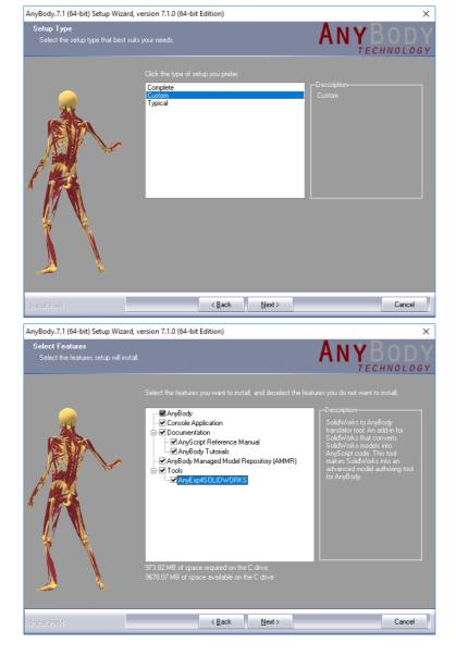
AnyExp4SOLIDWORKS requires a separate license, which is typically located in the same file as your AnyBody license. Importing the license file into AnyBody through the license manager will place the file in the proper location for AnyExp4SOLIDWORKS to find it.
