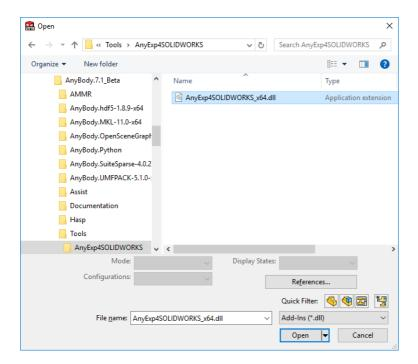
The AnyExp4SOLIDWORKS DLL can be found in the AnyBody installation, typically in the folder "C:\Program Files\AnyBody Technology\AnyBody.X.X\Tools\AnyExp4SOLIDWORKS", where X.X indicates the AnyBody version number.
